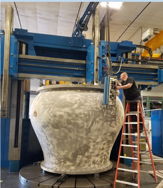
INDICATING DIFFUSER BOWL TO CHECK CONCENTRICITY OF REGISTERS AND MACHINE CASE RING FIT
