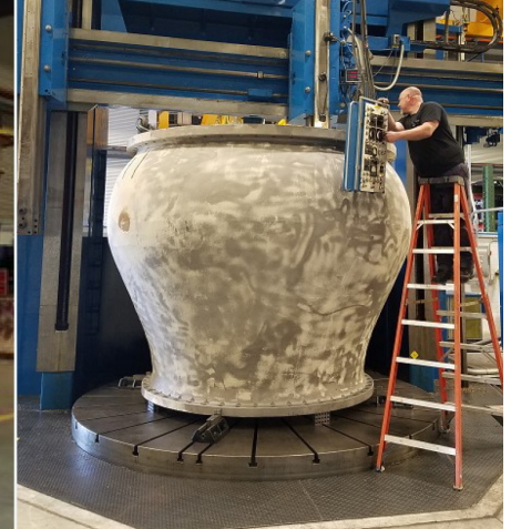
Indicating diffuser bowl to check concentricity of registers and machine case ring fit
