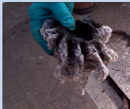
Material removed from a recess vane pump after 2-month test period
