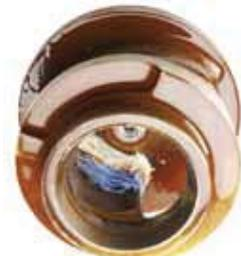
Figure 5: Accumulation in a single-vane impeller
