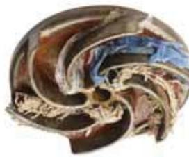
Figure 6: Accumulation in a vortex impeller
