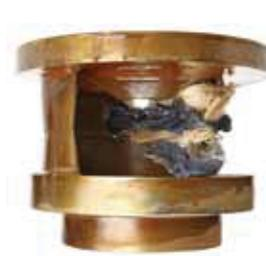
Figure 4: Accumulation in a single-vane impeller
