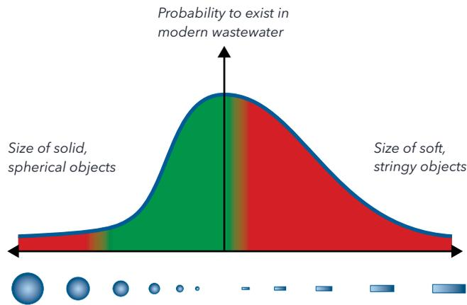
Figure 8 shows the types of solids that can pass through a traditional impeller with a large throughlet. The green area indicates objects with a high probability to pass through the pump. The red area indicates a higher probability of clogging.
