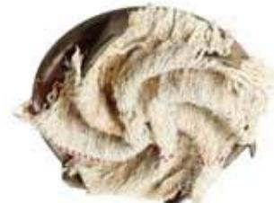
Figure 7: Accumulation in a vortex impeller
