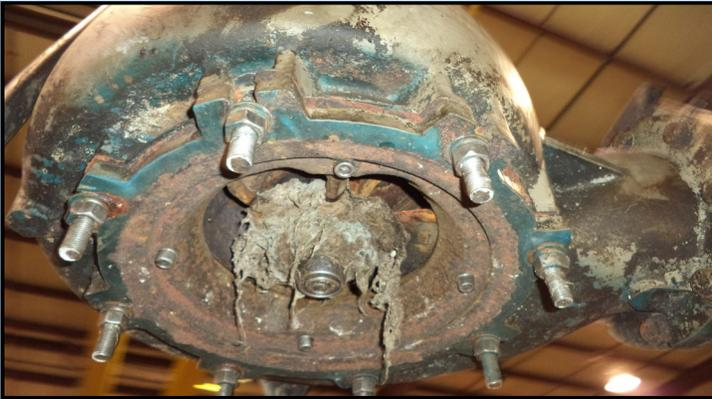
**Problem:** The Fawn River Lift Station is a duplex station that pumps on average 40 million gallons of sewage per month to the City of Sturgis Wastewater Treatment Plant. The station had been in service for only 6 years when one of the Hayward Gordon CHOPX8BS chopper pumps suffered a catastrophic failure, leaving only one pump in operation. WWTP personnel recognized that operating on one pump was not an option, and they needed both a short-term and long-term solution to the problem.
